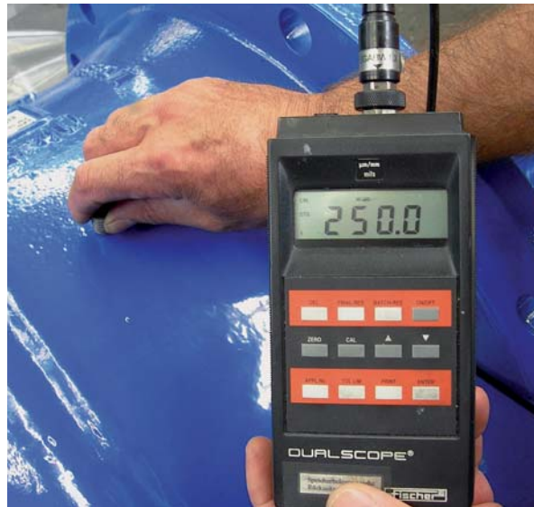
Fig. 3: Coating thickness test on a VAG EKN® Butterfly Valve
