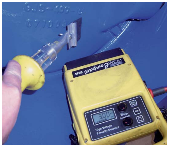
Fig. 4: Porosity testing the coating on a VAG EKN® Butterfly Valve
