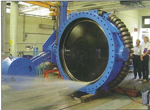
(f) The EKN DN 2000 butterfly valve for the right bottom outlet is opened slowly at a water pressure of 7 bar, during the factory leakage test.
